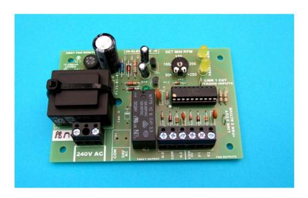
This module allows remote monitoring of one or two fans. It provides a set of voltage free relay change over contacts which operate if a fan fault is detected.
